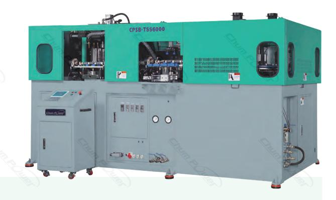
To improve safety and durability, the sensor system has been upgraded for better detection accuracy and stability. An added mold-closing sensor ensures correct toggle positioning and boosts overall safety.
